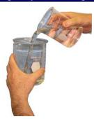
PSF-5cSt Silicone Bath Fluid is a low viscosity 100% PDMS silicone that has a service temp range of -70°C to 150°C closed system.
